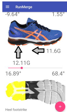
Figure 2: Side view (top) and bottom view (bottom) of the shoe. Pronation and stance angles are visible, as well as Gs values and footstrike colouration.
