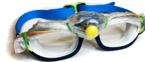
Figure 3: VOS prototype. The electronics are enclosed in a waterproof bag and attached to the swimming goggles with elastic bands.
